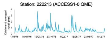
Figure 3 Example runoff time-series from station 222213 at Suggan Buggan River in the Snowy River Catchment (based on AWRA simulation using ACCESS1-0 and bias corrected using the QME bias correction method).
