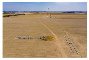
Figure 2 Damage to the Mortlake to Moorabool to Heywood interconnector from the 31 January 2020 event. (Source: AusNet)
