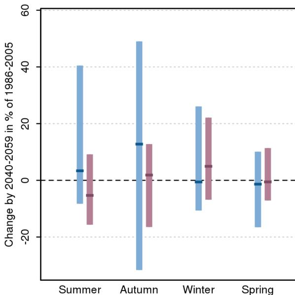
Figure 4. Projected percentage change in the 1-in-20 year maximum daily rainfall 2040-2059 compared to the 1986-2005. Blue bars (left): medium emissions. Purple bars (right): high emissions. Dark horizontal lines: median.
