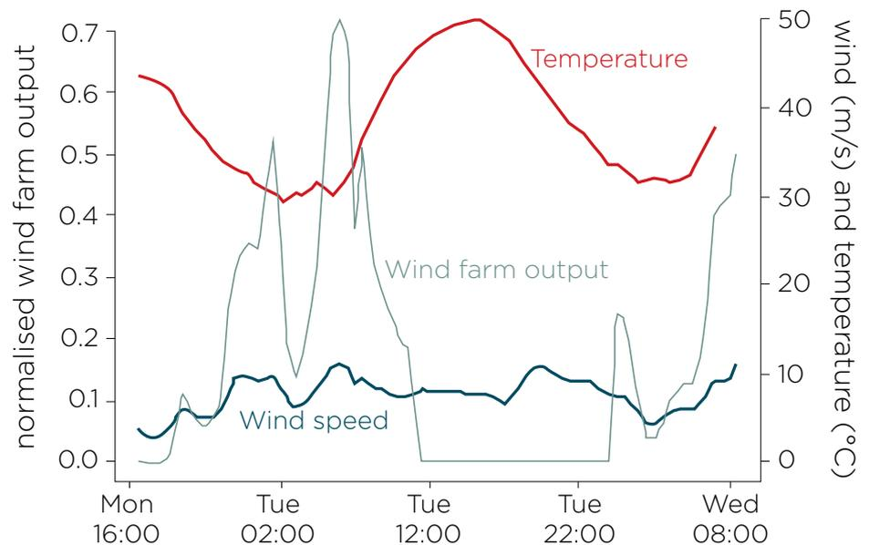
Figure 5 Thirty-minute simulation of wind farm output (black line) for varying temperature (red line) and wind speed (blue line) in Western Victoria.
