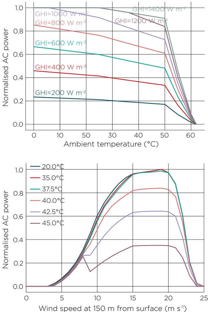
Figure 2 Indicative power conversion models used in this case study: Solar farm output (top) as it varies with temperature (horizontal axis) and Global Horizontal Irradiance (GHI, coloured lines). The wind farm model (bottom) describes output varying with wind speed (150 m from surface; m s<sup>-1</sup>, horizontal axis) and temperature (coloured lines).
