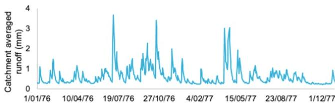
Figure 3 Example runoff time-series from station 222213 at Suggan Buggan River in the Snowy River Catchment (based on AWRA simulation using ACCESS1-0 and bias corrected using the QME bias correction method).
